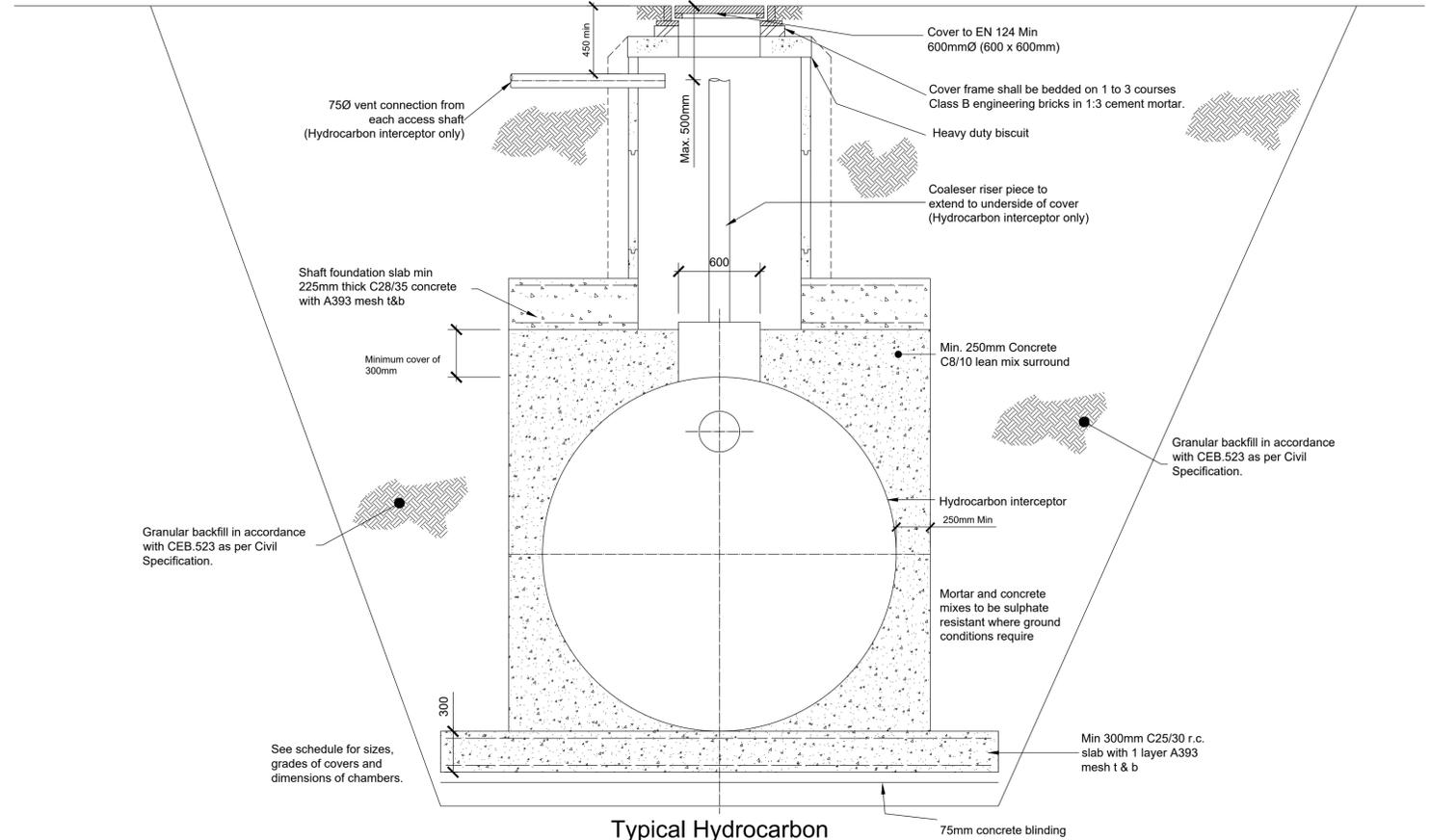
**Typical Hydrocarbon Interceptor Installation Detail**
